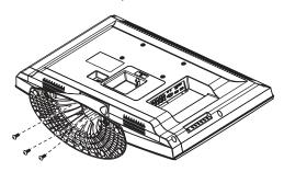
3 Secure the wall mount bracket to the back of your TV using the four M4 screws provided with the bracket. Screw length should not be over 11 mm.
